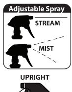
Always Turn spray tip clockwise to off when not using to prevent leaking.
